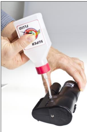
Fig. 17: Suction of the excess fluid
